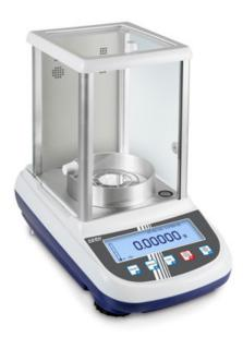
**KERN ALJ 200-5DA** with optional ionisor **II**, see Accessories. High-precison semi-microbalance. Thanks to its precison, this model is suitalbe to calibrate pipettes.
